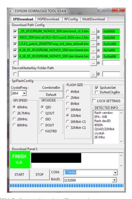
After flashing the ESP it finally started to reply to AT commands.
