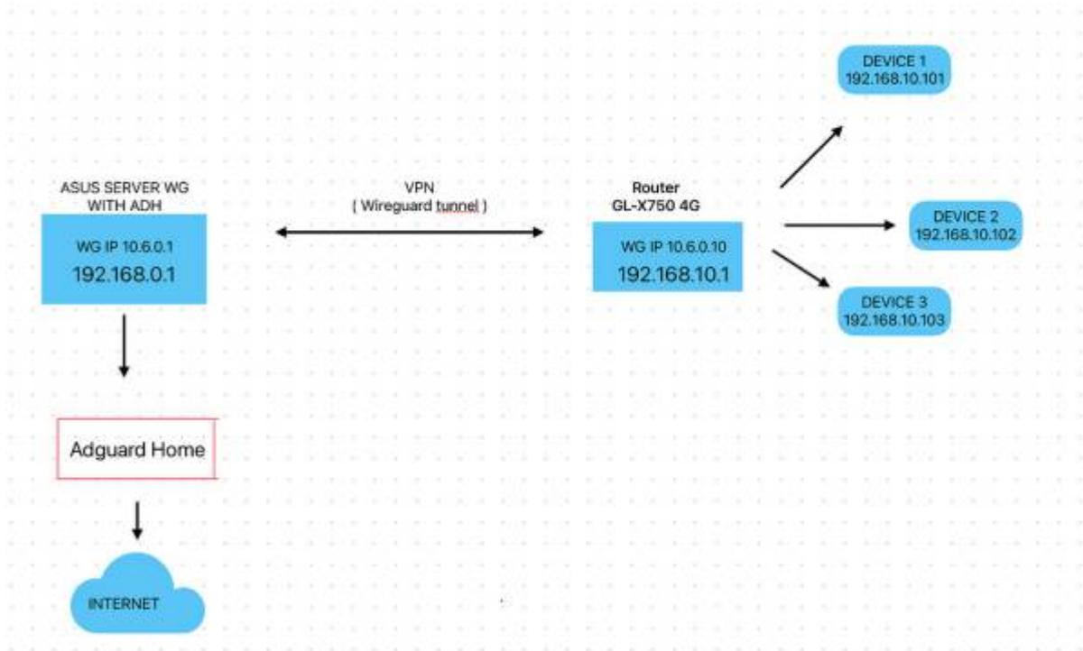
Our solution bases on the GL router, including the VPN Server and Client. Only for reference.
